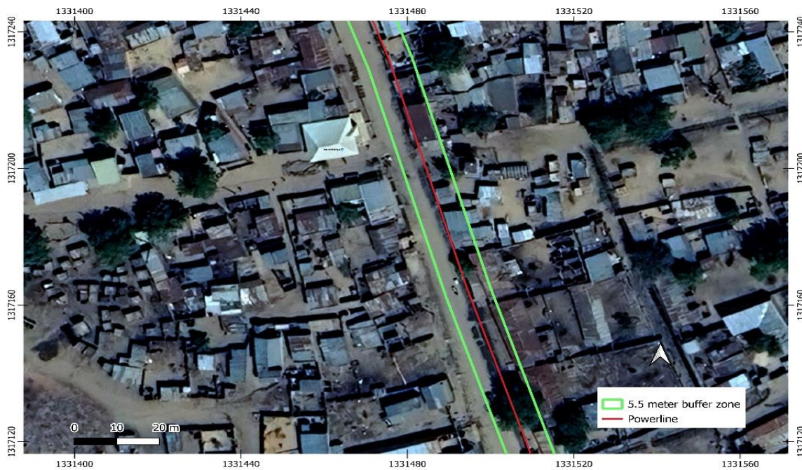
Figure 4: Encroached Structures Within the 5.5 m Buffer Zone of the 33 kV Powerline at Bayan Tasha
