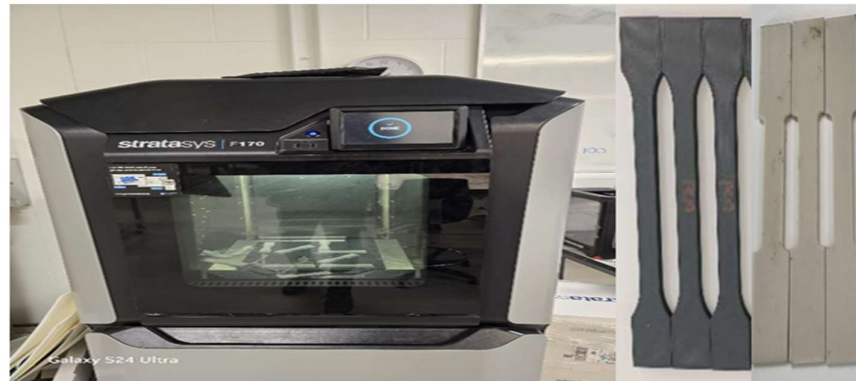
Figure 1.(a) Stratasys F170printer. Test specimen design; (b)visual presentation
